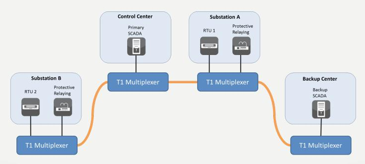
Figure 1: Linear Add/Drop T1 network carrying SCADA/RTU and Protective Relaying
